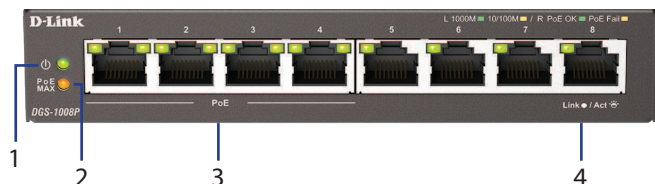
Figura 1: LED del panel frontal
