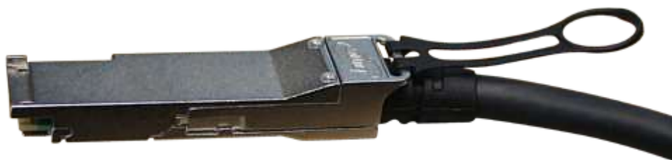
Figure 7-12 QSFP+ cable plug
