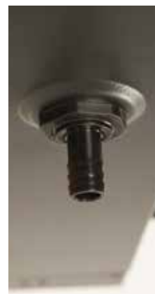
Condensation-water discharge fittings
