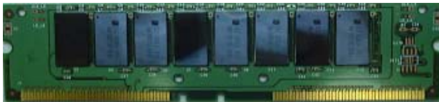
Figure 1: RIMM Module shown with heat spreader removed
