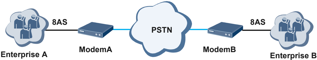
Figure 4-79 Connecting enterprises through modems
