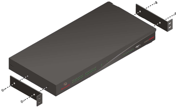
Figure 2.4: AMX5000 Switch Rack Mounting Diagram
