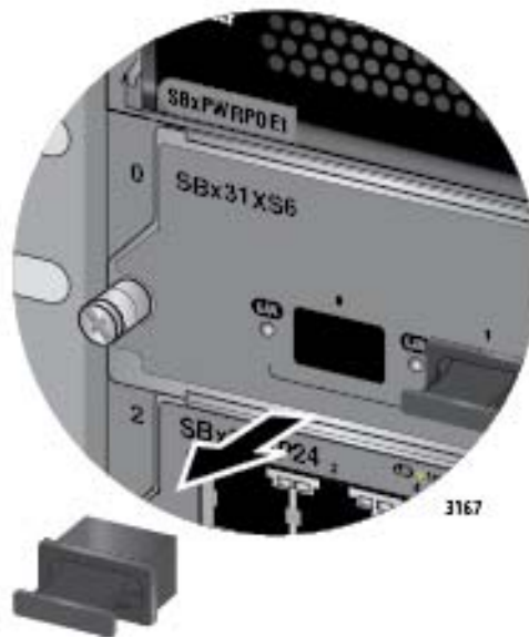
Figure 92. Removing a Dust Cover From an SFP+ Slot in the AT-SBx31XS6 Line Card
