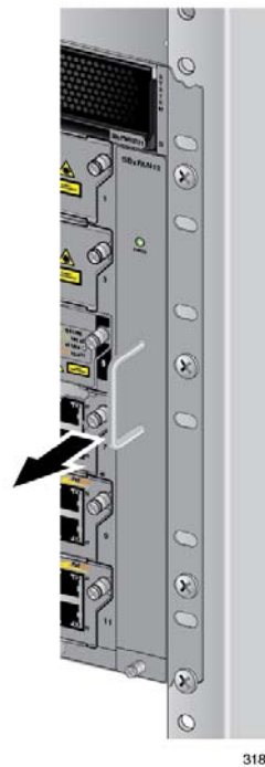
Figure 162. Loosening the AT-SBxFAN12 Fan Module from the Backplane Connector
