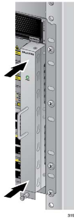
Figure 166. Securing the AT-SBxFAN12 Fan Module on the Backplane Connector
