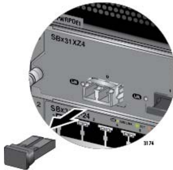
Figure 102. Removing the Protective Cover from an XFP Transceiver in the AT-SBx31XZ4 Line Card
