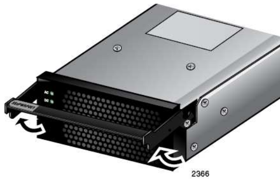
Figure 55. Raising the Handle on the AT-SBxPWRPOE1 AC Power Supply
