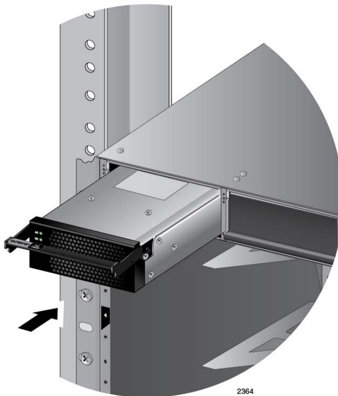
Figure 56. Inserting the AT-SBxPWRPOE1 AC Power Supply
