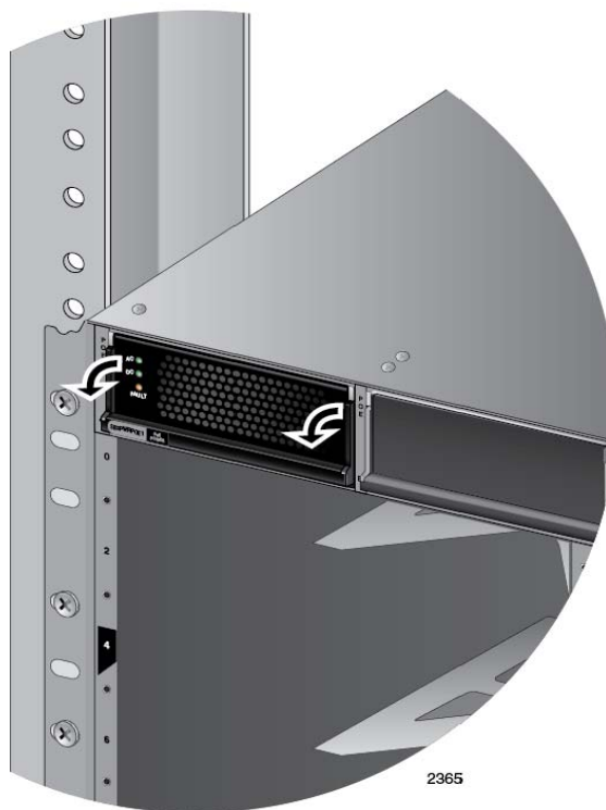
Figure 57. Locking the Handle on the AT-SBxPWRPOE1 AC Power Supply
