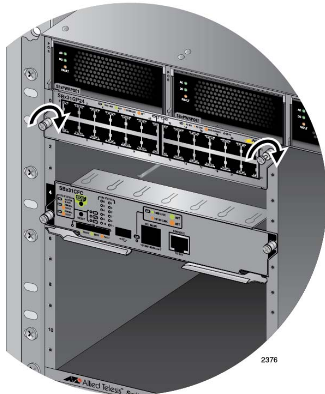
Figure 77. Tightening the Thumb Screws on an Ethernet Line Card
