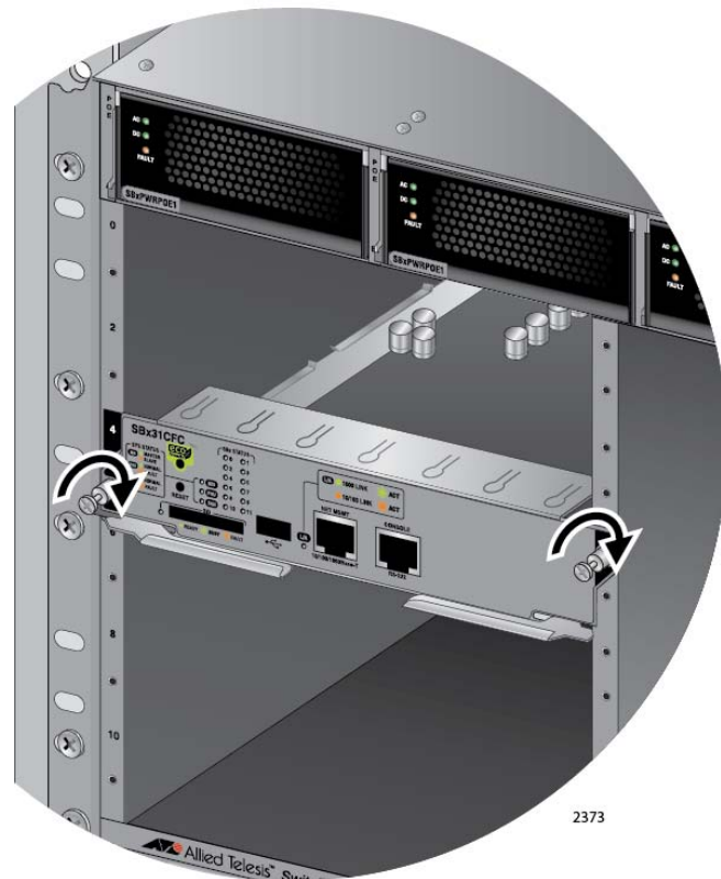
Figure 72. Tightening the Thumb Screws on the AT-SBx31CFC Card
