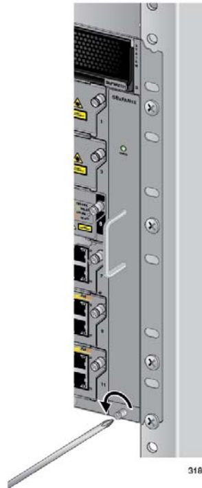
Figure 161. Loosening the Screw on the AT-SBxFAN12 Fan Module
