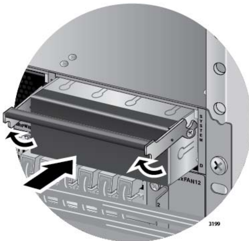
Figure 148. Installing a Blank Power Supply Slot Cover
