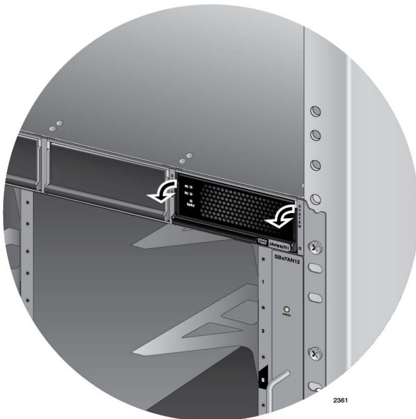
Figure 52. Lowering the Handle on the AT-SBxPWRSYS1 or AT-SBxPWRSYS2 AC Power Supply
