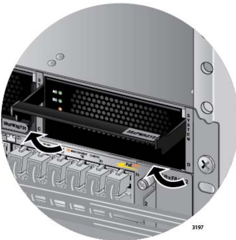
Figure 146. Lifting the Locking Handle on the Power Supply
