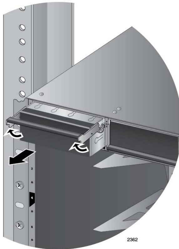
Figure 53. Removing the Blank Slot Cover from Power Supply Slot A
