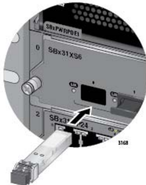
Figure 94. Installing an SFP+ Transceiver in the AT-SBx31XS6 Line Card
