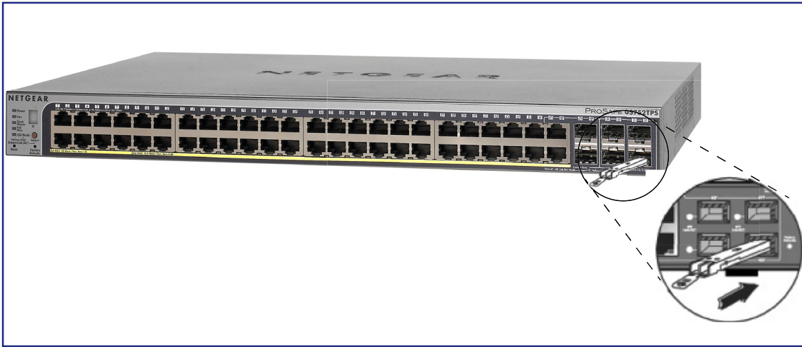
Figure 14. Installing and SFP Transceiver Module (GS752TPS Shown)
