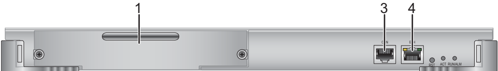
Figure 6-7 Ports on the ES0D00SRUA00 panel
