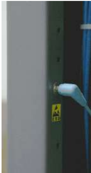
Figure 2-7 ESD jack on the N66E cabinet
