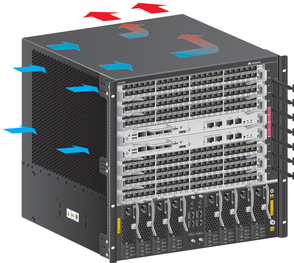
Figure 3-24 Airflow in the S7706 chassis
