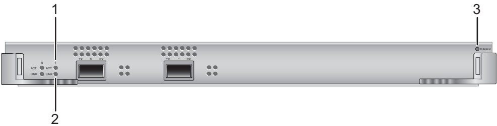
Figure 6-124 Indicators on the ES1D2L02QFC0 panel
