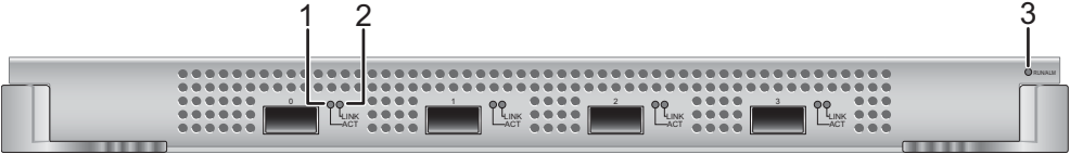
Figure 6-106 Indicators on the ES0D0X4UXA00, ES0D0X4UXC00/ES1D2X04XEC1, or ES1D2X04XED0 panels
