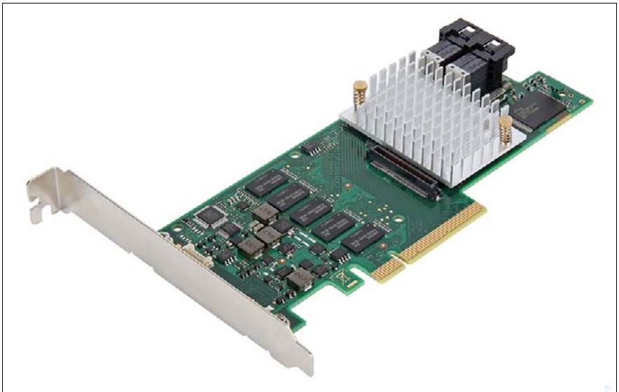
Figure 23: "PRAID EP400i / EP420i" (based on LSI SAS3108)
