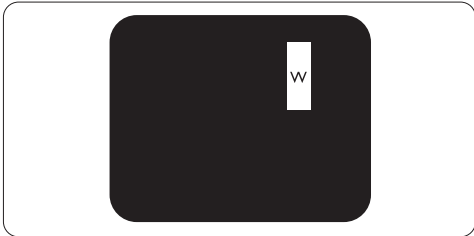
Three adjacent lit sub pixels (one white pixel)
