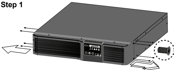
Figure 8 Convert the Liebert PSI for rack installation
