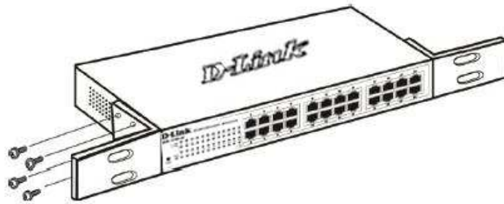
Figure 6 – Attach the mounting brackets to the Switch
