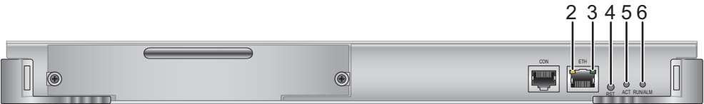
Figure 6-5 Indicators on the ES0D00SRUA00 panel
