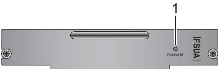
Figure 6-15 Indicator on the ES0D00FSUA00 panel
