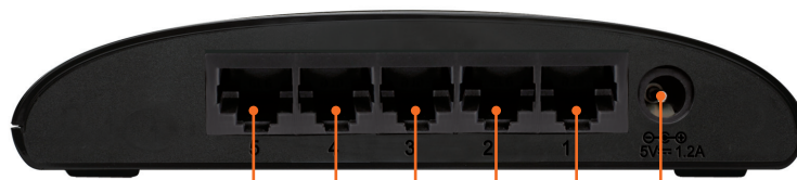
5 RJ-45 10/100 BASE-TX PORTS Connects to computers, print servers, or network storage
