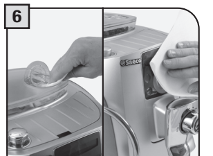
Clean the pre-ground bypass doser with a dry cloth. Wipe the display.
