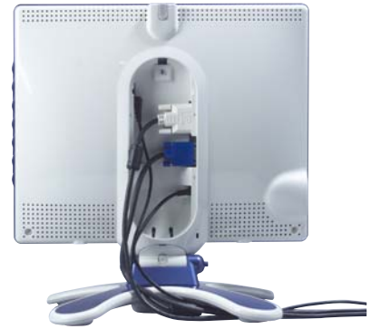
Monitor showing all cables in place
