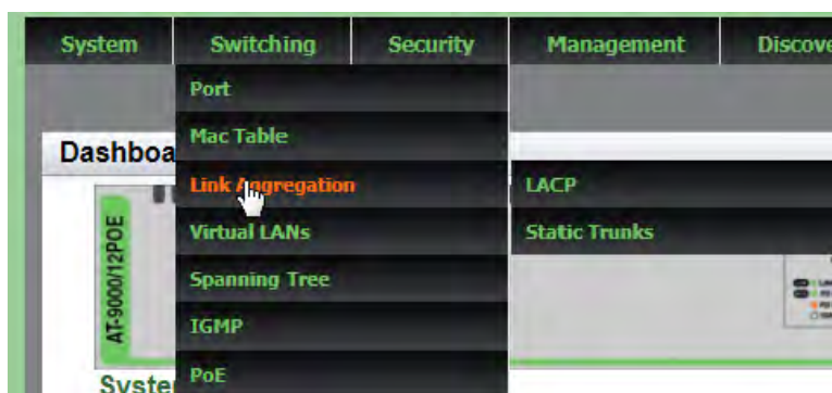
Figure 42. Switching Tab with Link Aggregation Selected
