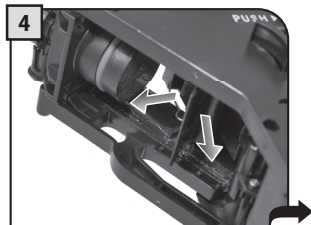
Apply the lubricant evenly on both side guides.
