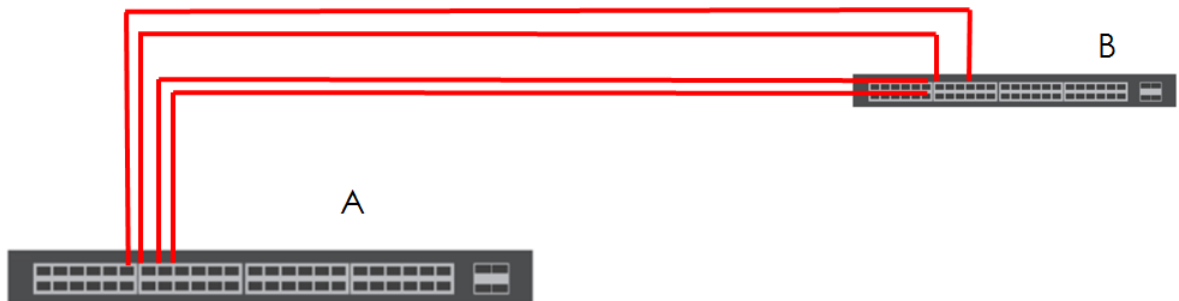
Figure 114 Trunking Example - Physical Connections
