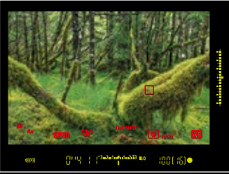
All display – AF point, shooting, electronic level information, and more can be reviewed on the viewfinder.
