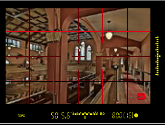
Grid display – Useful for scenes where horizontal or vertical lines are stressed, such as architecture.
