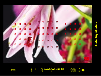
Single-spot point AF display – Focuses on a smaller area for precise focus on small subjects.
