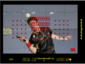
Zone AF (9 patterns) display – The AF points are divided into five focusing zones, useful for off-center shots.
