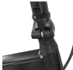
Rotate the fastening lever from to prevent the accidentally unlocking.
