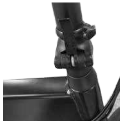
Close the lock lever pushing upwards
