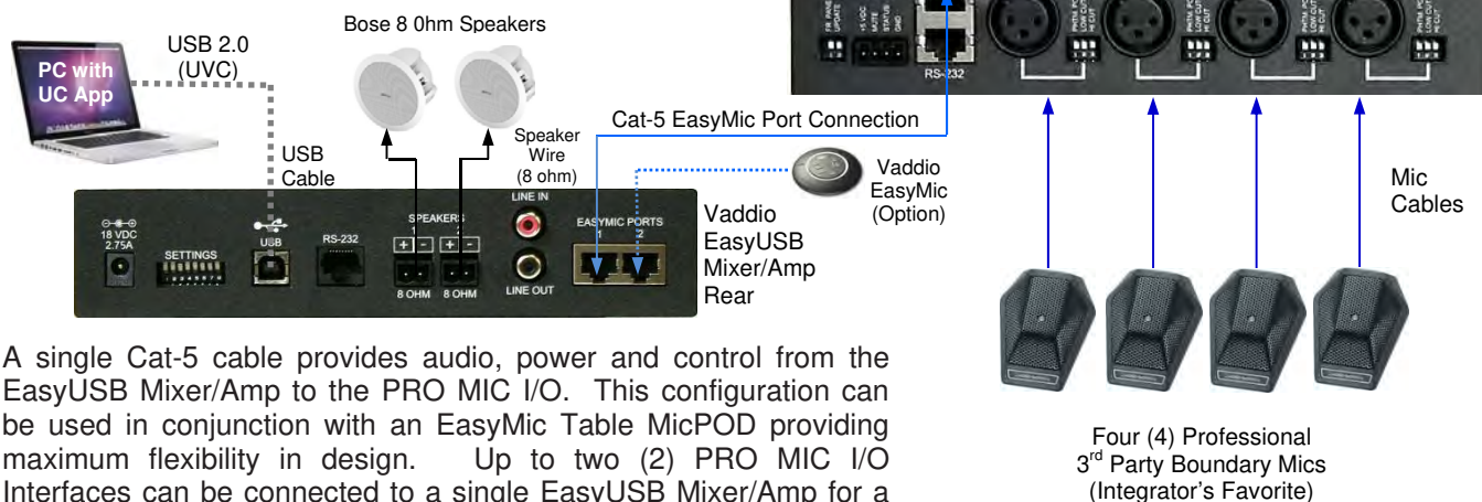
Diagram: PRO MIC I/O 4-Mic Configuration with
