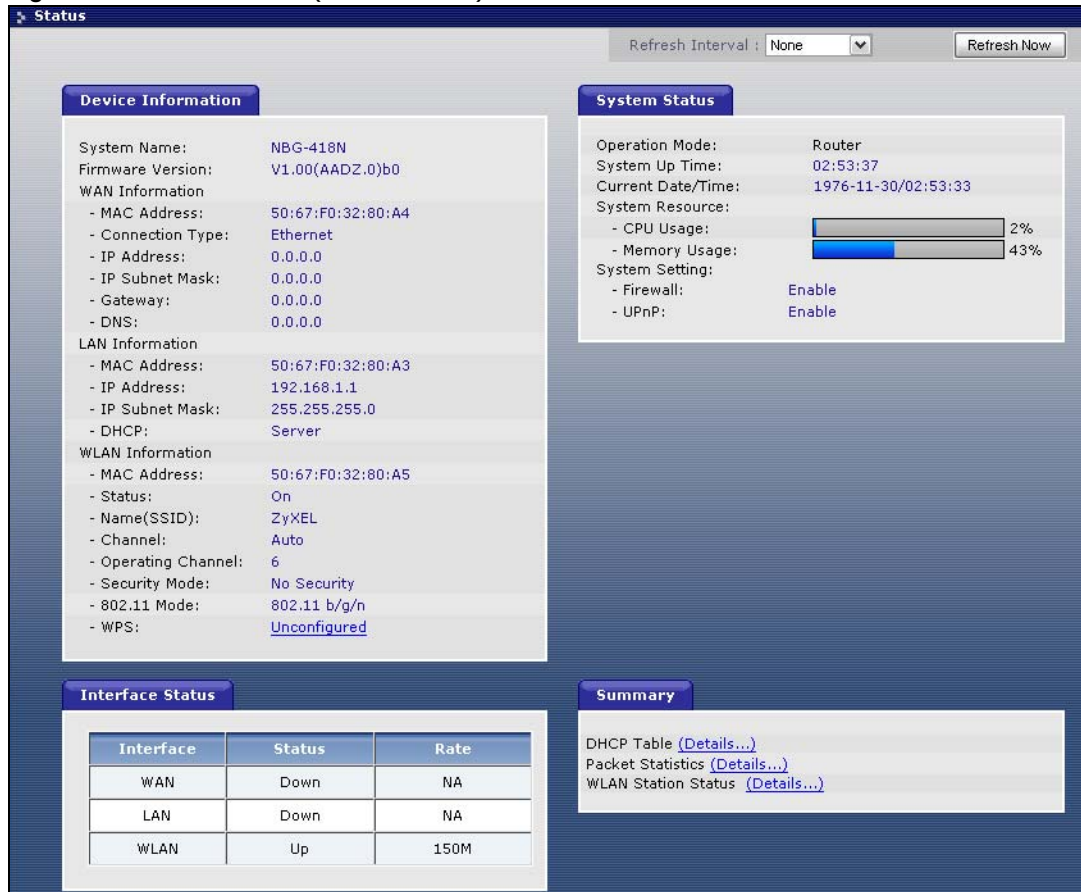
Figure 25 Status Screen (Router Mode)
