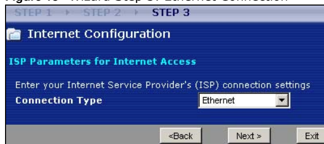
Figure 13 Wizard Step 3: Ethernet Connection
