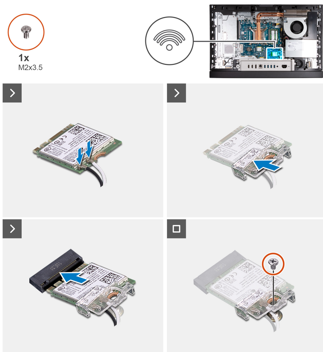
Figure 29. Installing the wireless card
