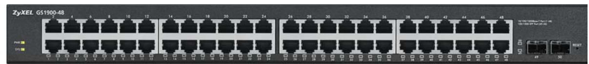
Figure 16 Front Panel: GS1900-48
