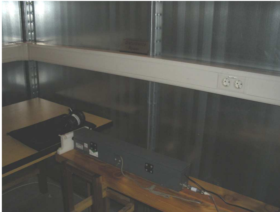
Photograph 3: Set-up for measurement of disturbance power
