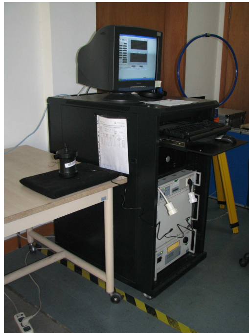
Photograph 2: Set-up for measurement of disturbance voltage
