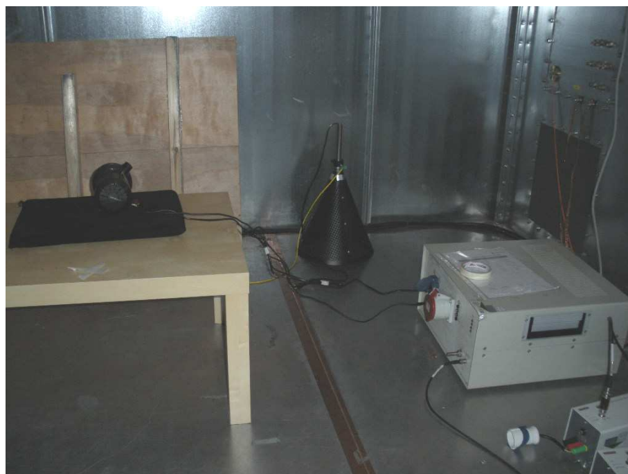
Photograph 2: Set-up for measurement of disturbance voltage
