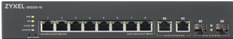
Figure 11 Front Panel: GS2220-10HP
