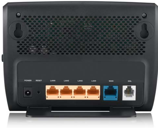
Figure 11 VMG3312-T20A Rear Panel
