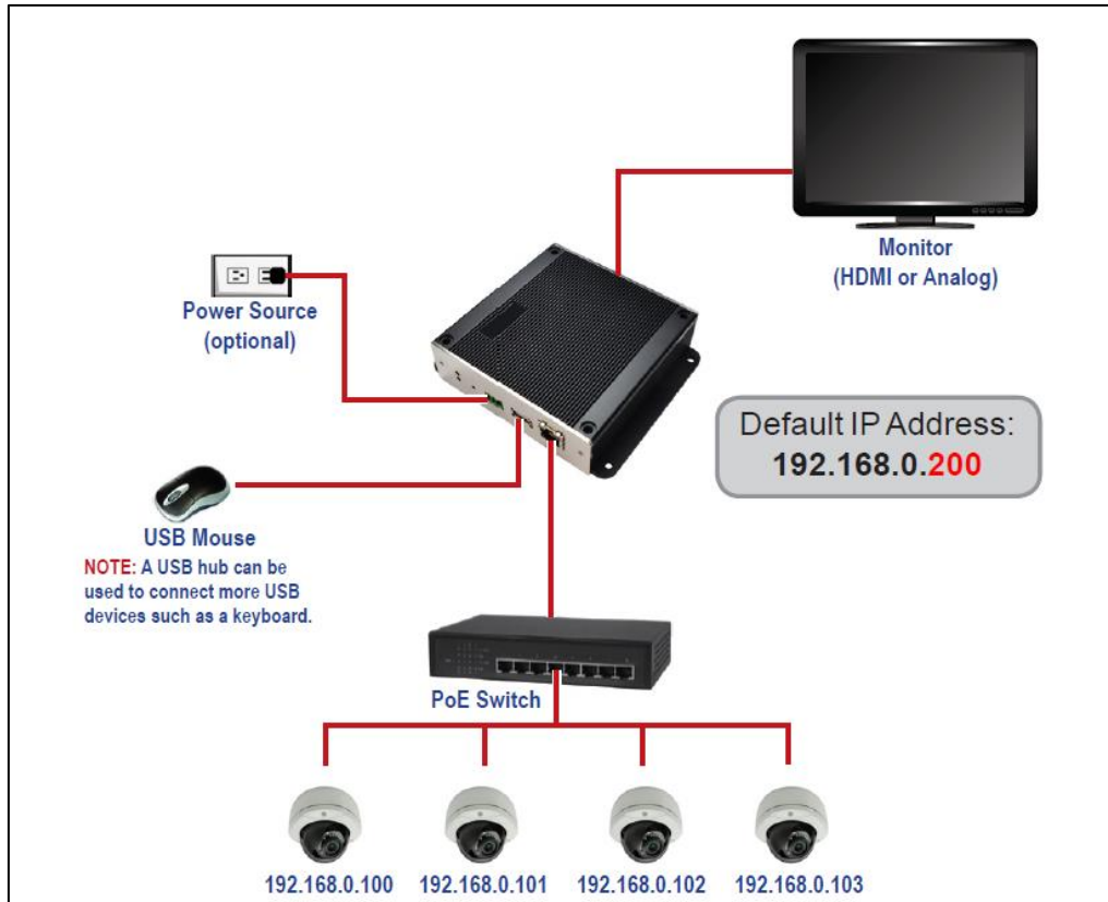
Local Area Network Connection Architecture
