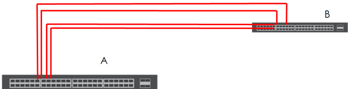
Figure 127 Trunking Example - Physical Connections
