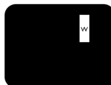
Three adjacent lit sub pixels (one white pixel)
