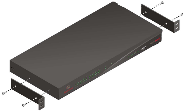
Figure 2.4: AMX5000 Switch Rack Mounting Diagram
