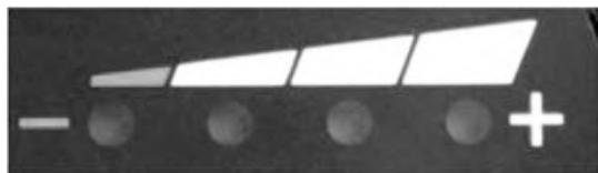
Battery power levels
