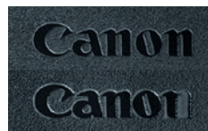
Logo on the genuine battery (top) and the counterfeit battery (bottom)
