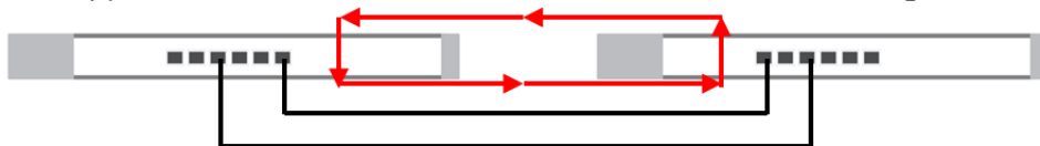
Figure 32 Two Connections between Switches Without Using the Spanning Tree Protocol (STP)
