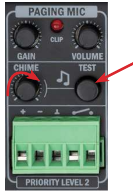
Figure 12. Paging Mic Adjustments
