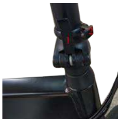
Close the lock lever (1) pushing upwards
