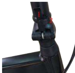
Rotate the safety ring (2) to prevent the fastening lever (1) from accidentally unlocking.
