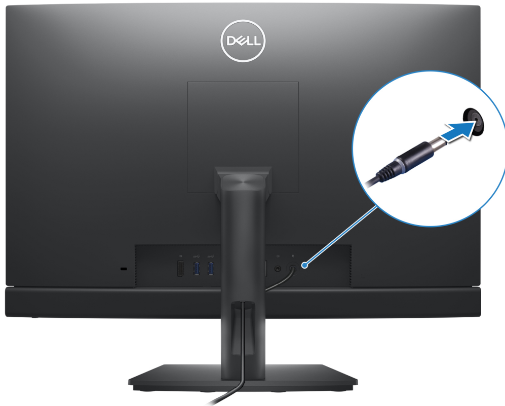
Figure 12. Connecting the power-adaptor cable
