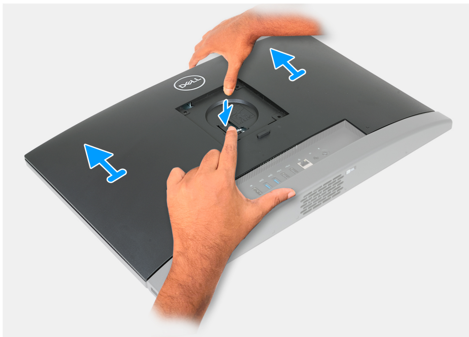
Figure 82. Removing the back cover
